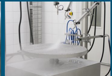
IPX9K - Flat spray nozzles
