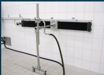
Hosedown according to UL 50E
